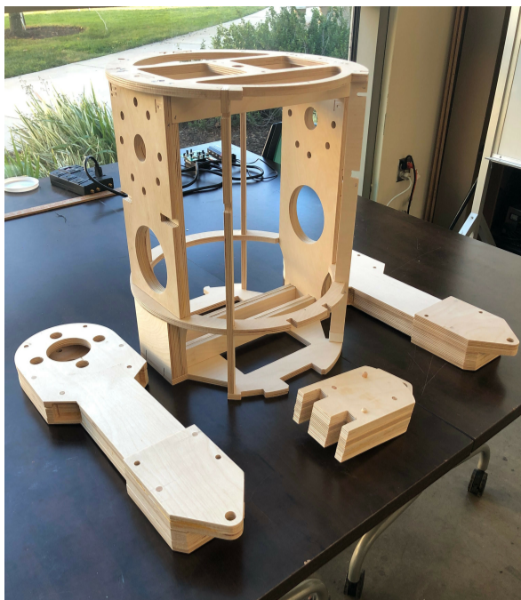
Fig. 2: Photograph of the student-assembled wood frame and wood legs. The diameter of the cylindrical main body is approximately 46 centimeters.
