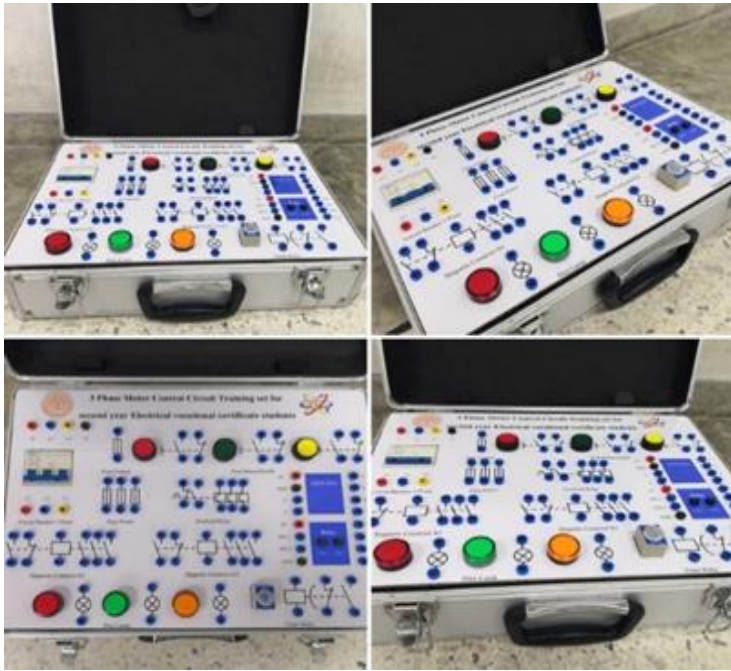
Fig 2. Three phase motor control circuit operating set
