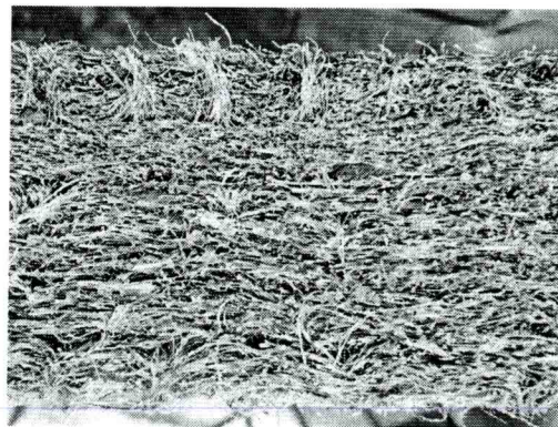
Figure 21 The insertion of natural latex in indoor acoustic and thermal insulation board
