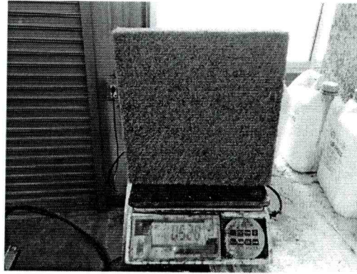
Figure 16 Density test of the indoor acoustic and thermal insulation board
