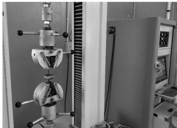
Fig. 5: Tensile strength perpendicular to the surface test of cement board
