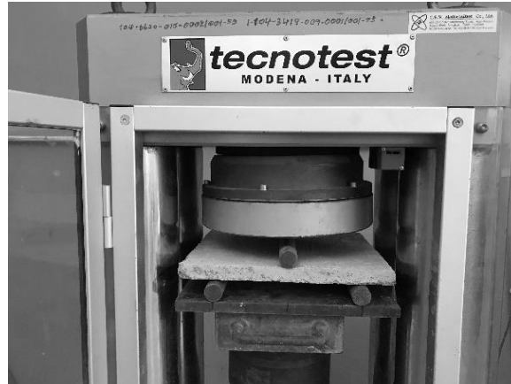
Fig. 4: Bending strength test of cement board
