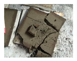
**Figure 6** Non-rigid of cement board mixed with Ground coffee as ratio 1:0.15 was cured 7 days.
