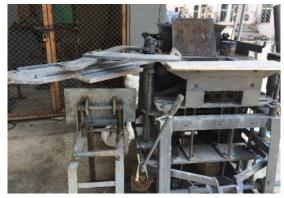
**Figure 2** The vibratecement board compressorfor molding the cement board.
