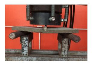
**Figure 4** Testing bending strength and modulus of elasticity of cement board from ground coffee.
