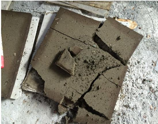
**Figure 6** Non-rigid of cement board mixed with Ground coffee as ratio 1:0.15 was cured 7 days.
