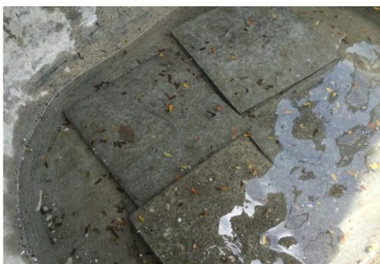
**Figure 3** Soaked cement boards from ground coffee for swell test.
