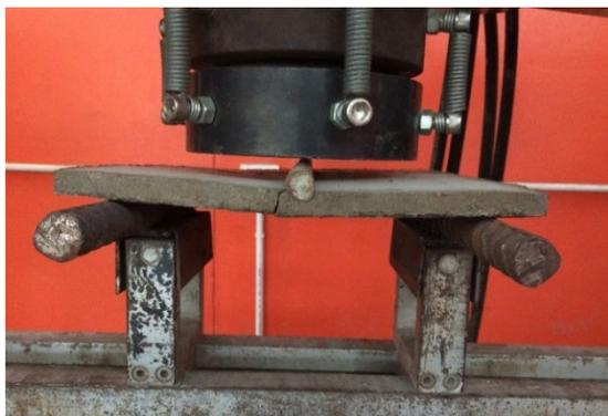
**Figure 4** Testing bending strength and modulus of elasticity of cement board from ground coffee.
