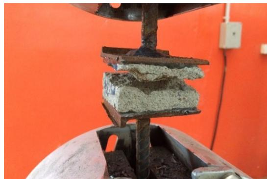
**Figure 5** Damage of test tensile strength at surface of cement board from ground coffee.
