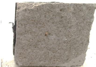
**Figure14** surface of cement board from ground coffee was damaged from tensile strength perpendicular with surface.
