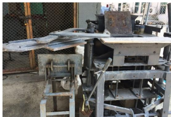
**Figure 2** The vibratcement board compressorfor molding the cement board.
